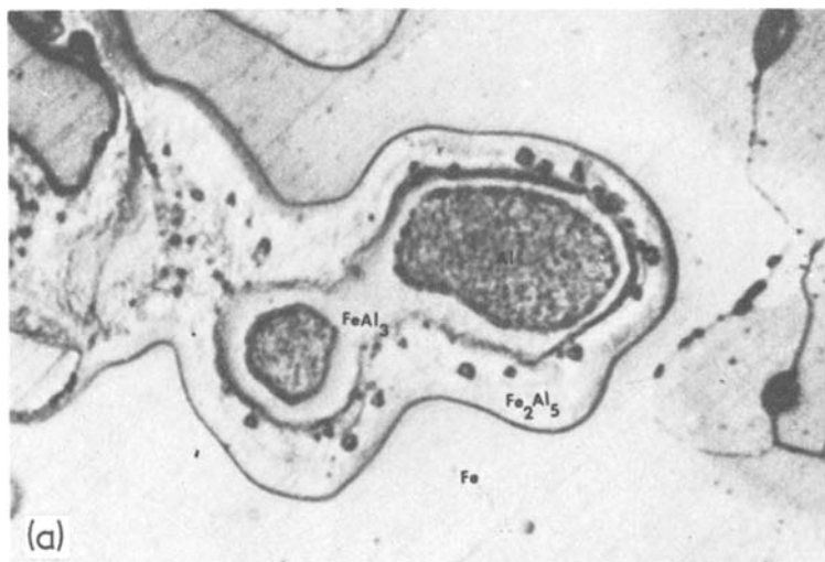
Figure 3 Optical micrographs of taper sections of the iron–aluminium interface; (a) specimen A, multi-phase “alloy” layer, (b) specimen B, single phase “alloy” layer. ( \times 300 ).
